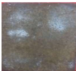
Fig. 17 Effect of time on corrosion morphology in immersion corrosion test specimens of uncoated and coated AZ91D Magnesium alloy
