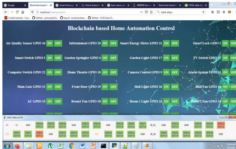
Fig. 4. This figure shows that if any of the device state is ON it changes the corresponding pin value to 1 in GPIO emulator. If any of the device state is OFF it changes the corresponding pin value to 0 in GPIO emulator.
