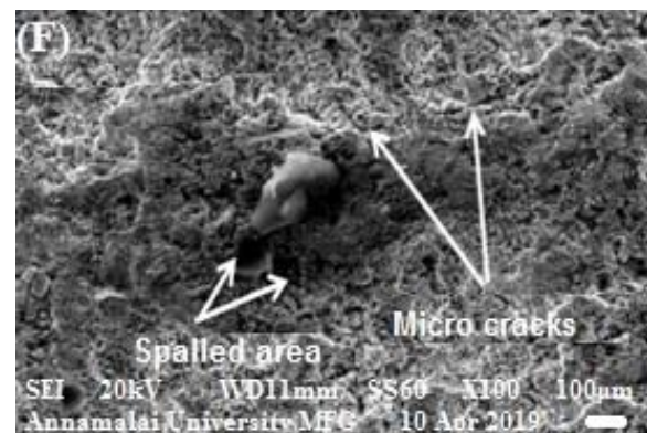
Fig. 9 SEM images of the eroded surface of substrate and coating at various water jet velocities
