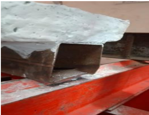
Figure-13: Buckling of hollow section support (CB2)
