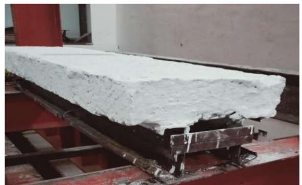
Figure -14: little Buckling of ISMC at at support (CB3)
