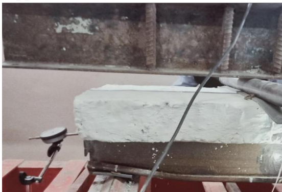
Figure-13: Buckling of hollow section support (CB2)
