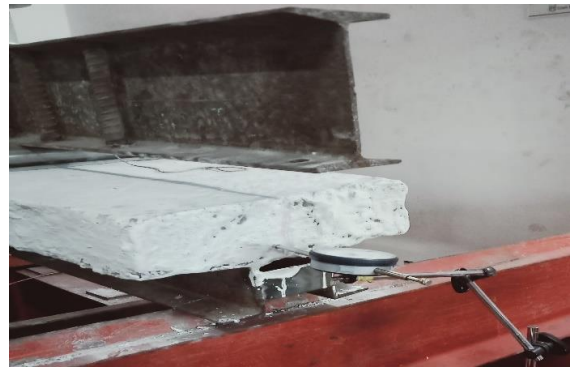
Figure -14: little Buckling of ISMC at at support (CB3)
