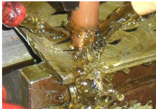
Figure 4 Flushing of dielectric during machining
