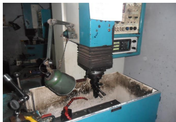
Figure 2 Spark EDM experimental setup
