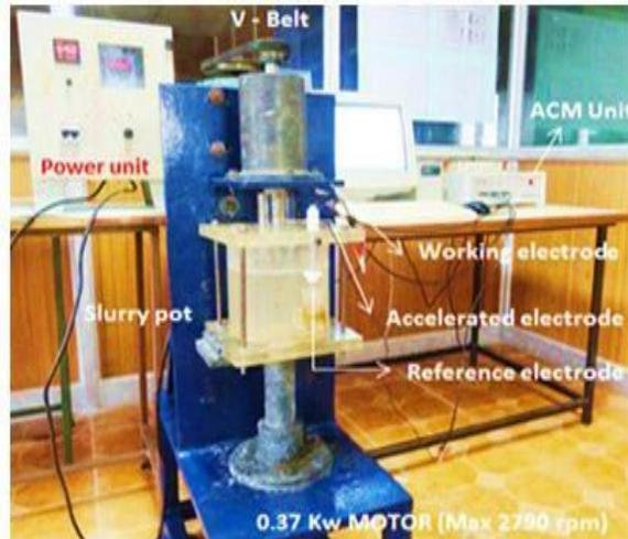
**Fig. 6 Pot type slurry erosion-corrosion tester**
