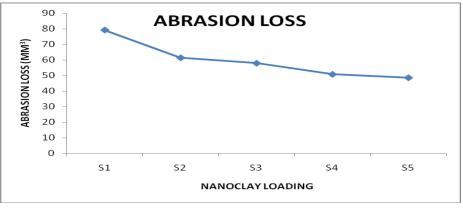
Figure 8.5 Abrasion loss of the EPDM/NBR composites
