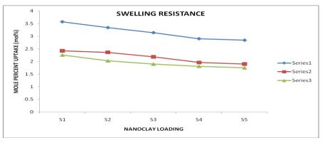
Figure 8.6 Swelling resistance (in terms of mole percent uptake) of the EPDM/NBR composites: Series 1 (Toluene solvent), Series 2 (pentane solvent) and Series 3 (carbon tetrachloride)
