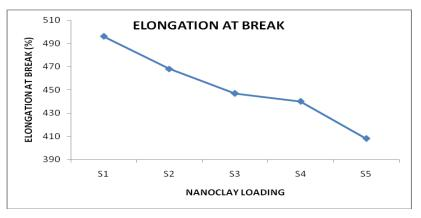
Figure 8.2 Elongation at break of the EPDM/NBR composites
