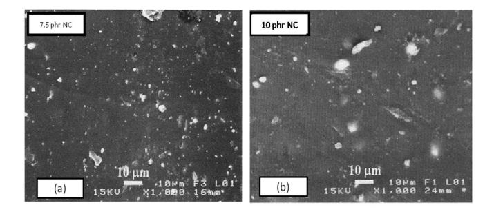
Figure 8.7 SEM micrographs of EPDM/NBR composites
