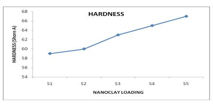
Figure 8.3 Hardness of the EPDM/NBR composites
