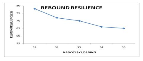
Figure 8.4 Rebound resilience of the EPDM/NBR composites
