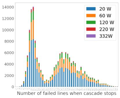
Figure-5: Number of failed lines in each category at steady state
