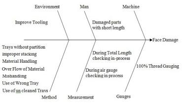
Figure No.4.2 Fish Bone diagram for the listed causes
